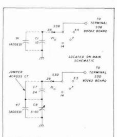
fig. 2. Modification of the receiver section of the Argonaut 509 requires minor additions to components switched by S3B and S3D.
